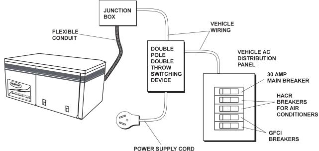
Figure 2.14 - Transfer Switch Isolation Method
